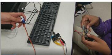
Away from home and want to feed your pet? Gabrielle and McKenzie code a microprocessor to send a remote radio signal to activate the servo motor to open the door, releasing the food.
