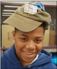
Wearable Technology. Going for a jog late at night? Malachi coded his processor to sense light levels in the environment and respond with a logical algorithm. He coded a microprocessor and fastened it to one of his teacher's old hats with a battery pack to test the prototype. Lights out? The warning, safety light comes on. Lights on? The warning light switches off!
